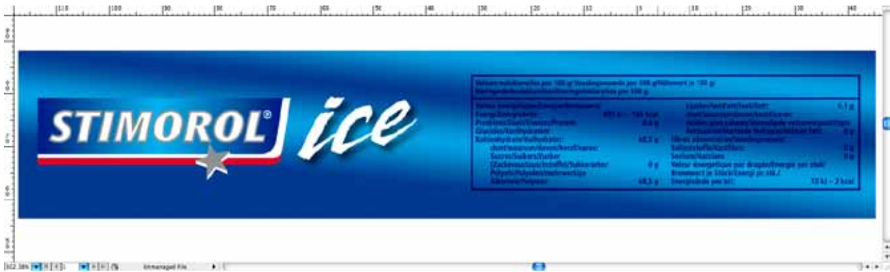
Design element that needs to be repeated on a seamless cylinder. The trim box, highlighted in blue, acts as the step and repeat reference cell.
