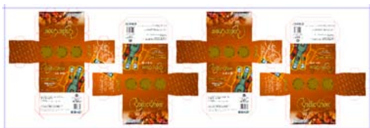
Automated layout based on MFG or CFF2 manufacturing files.
