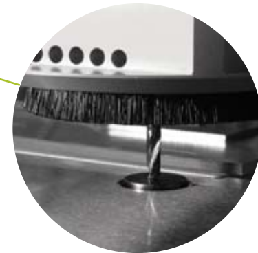
The Automatic Tool Leveling is a pressure sensitive pad that accurately and automatically calibrates the vertical operating level of all the Kongsberg XP tools.
